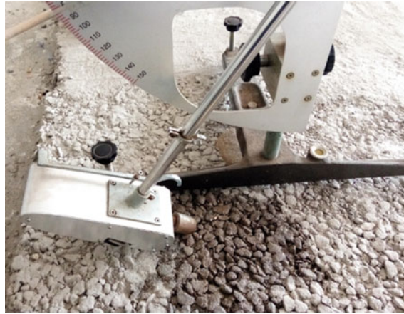
Fig. 6. Figure of pendulum friction coefficient test
