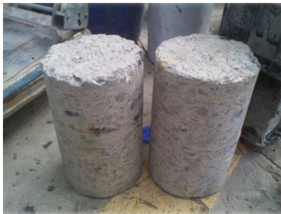
Fig. 2. Core sample figure of concrete pavement
