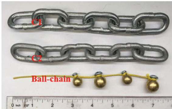
Fig. 2. Two steel link-chains and a ball-chain
