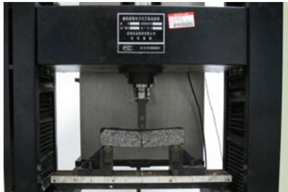
Fig. 3. The schematic of beam bending test
